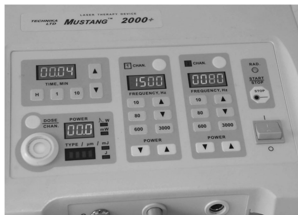
Figure 1 The laser apparatus used in this study (Mustang 2000+, Moscow, Russia) emitting at 810 nm.
